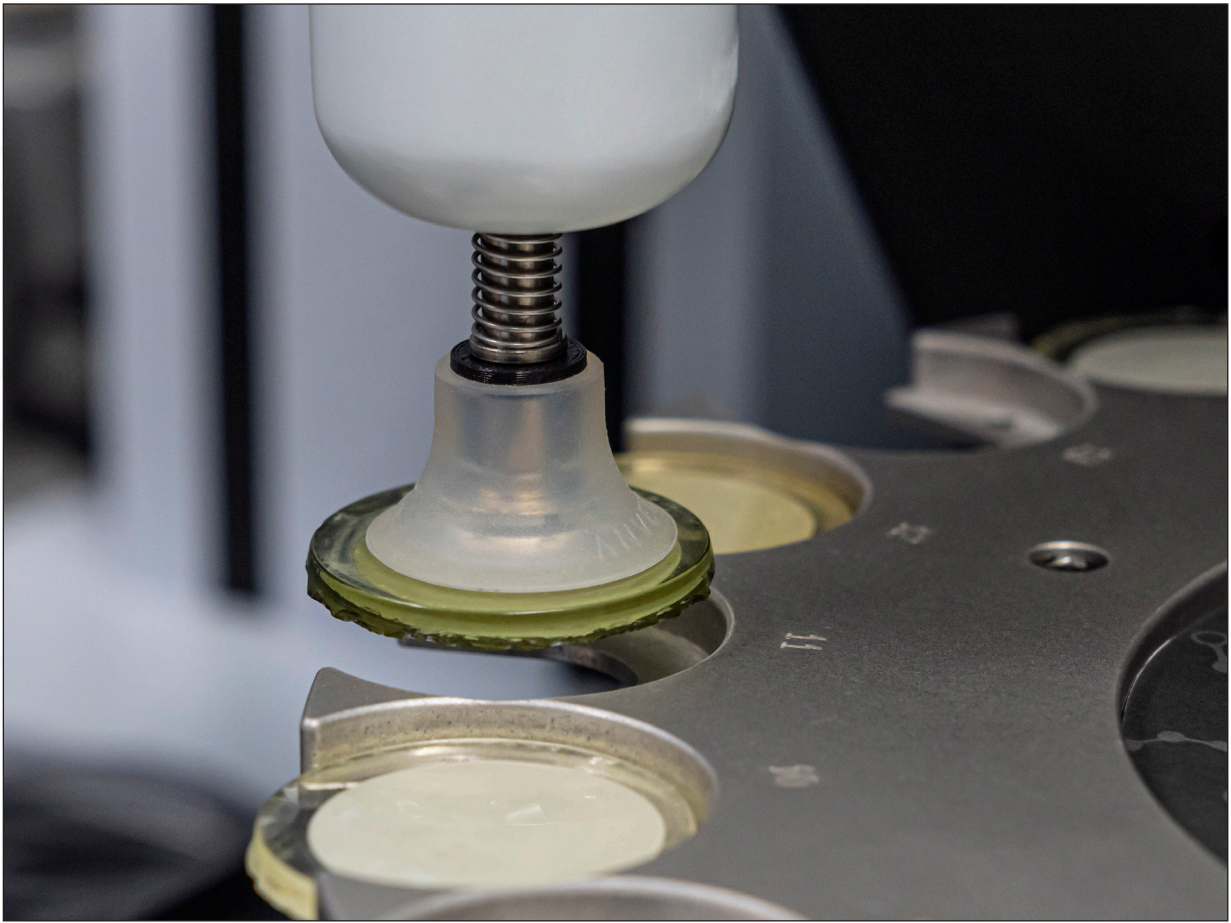
Figure 4. Samples loaded into Laser SC Carousel in preparation for analysis.
